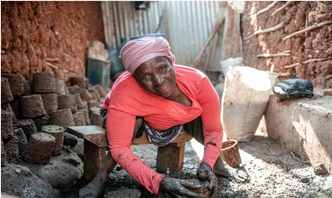
Mama Sarah makes briquettes from leftover charcoal dust in the informal settlements of Kibera, Nairobi.
